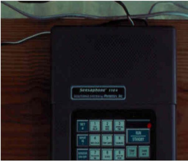
Figure 24. Alarm device that phones owner of deviations in set environmental parameters.
