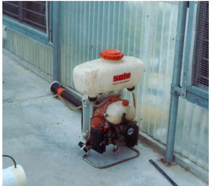
Figure 31. Motorized, backpack sprayer for applying pesticides.
